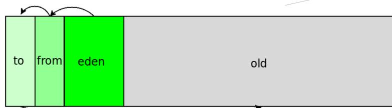
2-Gen(most common) Heap Layout
